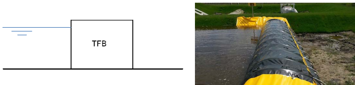
Figure 4-3 Schematic cross section of a theoretical Temporary Flood Barrier (TFB) (left) and a picture of a TFB (right) (source: www.tubebarrier.com )
