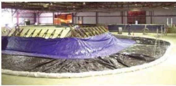
Figure 7: Example testing of a 'porta dam' using to the USACE guidelines for testing (Wibowo & Ward 2016)
