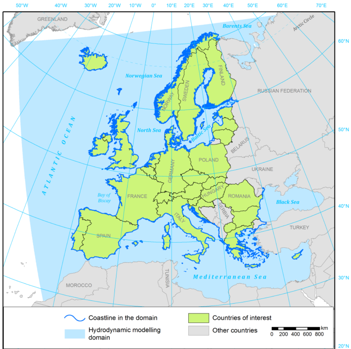
Figure A2. Domain used in RAIN project to obtain coastal flood hazard maps. Coastline geometry from CCM2 dataset (de Jager and Vogt 2010).
