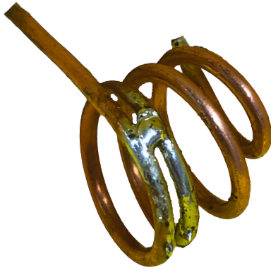
Figure 5.16: Coil used as inductor
