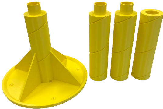
Figure 5.4: The four 3D printed parts submarine antenna
