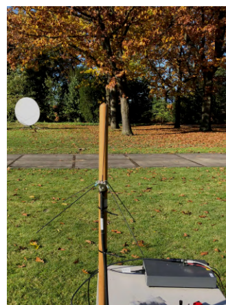
Figure 6.14: Transmitting antenna radiation pattern measurement outdoor
