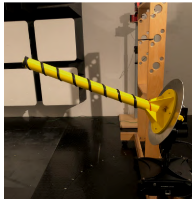
Figure 6.7: Submarine antenna during measurement
