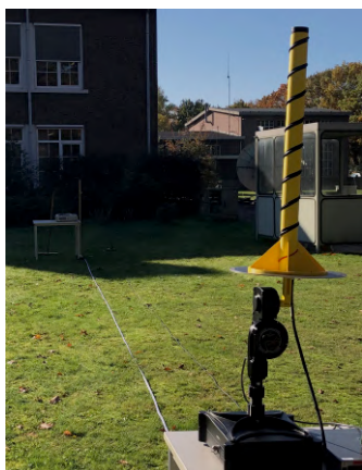
Figure 6.12: Radiation pattern measurement set-up outdoor
