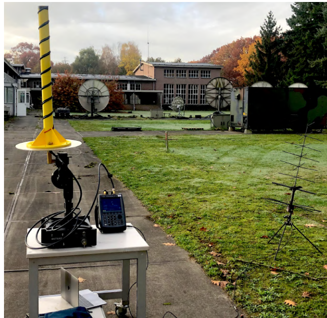
Figure 6.15: Outdoor measurement set-up for link strength testing
