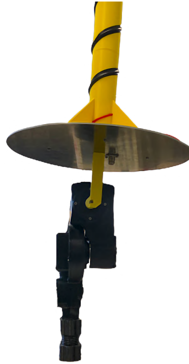
Figure 5.8: Connector on underside ground plane
