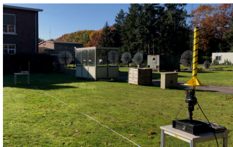
Figure 6.13: Radiation pattern measurement set-up outdoor
