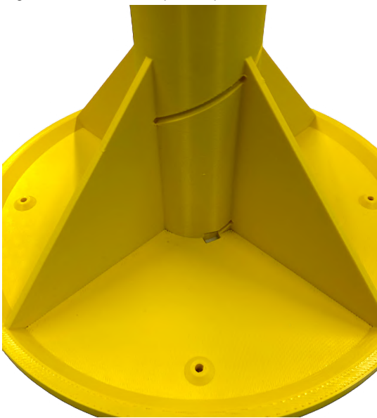
Figure 5.6: Connector hole in antenna base plate
