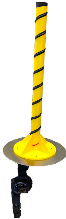
Figure 5.7: Assembled antenna on RRS stand
