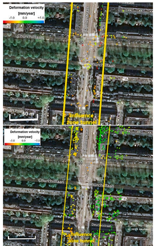
Fig. 9. InSAR points near Churchilllaan: (a) low points, on the ground surface. (b) high points, on the buildings. The colored dots indicate the vertical deformation rates in mm/y. The yellow lines indicate the influence zone of the tunnel.
