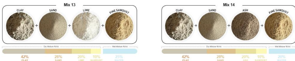
Figure 36 Refined Mixtures Composition Source: Author
