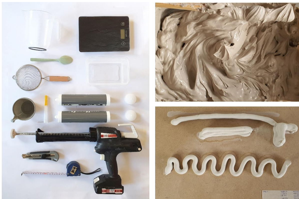
Figure 34 Tools Used for Extrusion Experiment, Example of Wet Mixture, Example of Dry Extrusions Source: Author
