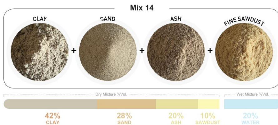
Figure 41 Final Mixture Composition Source: Author
