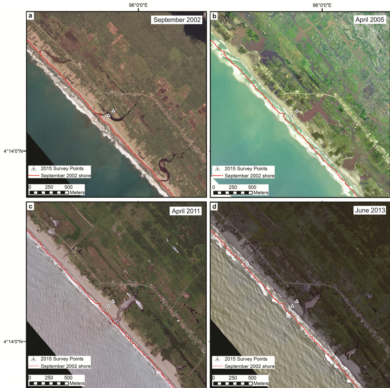
Figure 2: Detail of Figure 1b showing pre-tsunami conditions (i.e. 2002) and post tsunami coastal development. Red line marks 2002 shore in all images. Triangles indicate location of beach surveys (see Figure 3) and mark top of beach ridge and most seaward swale in 2015. April 2005 and 2011 images were taken towards the end of the East Monsoon season; 2002 and 2013 images during the more energetic West Monsoon. Satellite imagery is from Quickbird (2002), World-View-2 (2011) and Pleiades (2013). 2005 aerial photographs are from the SIM Center of the Aceh and Nias Rehabilitation and Reconstruction Board (BRR).
