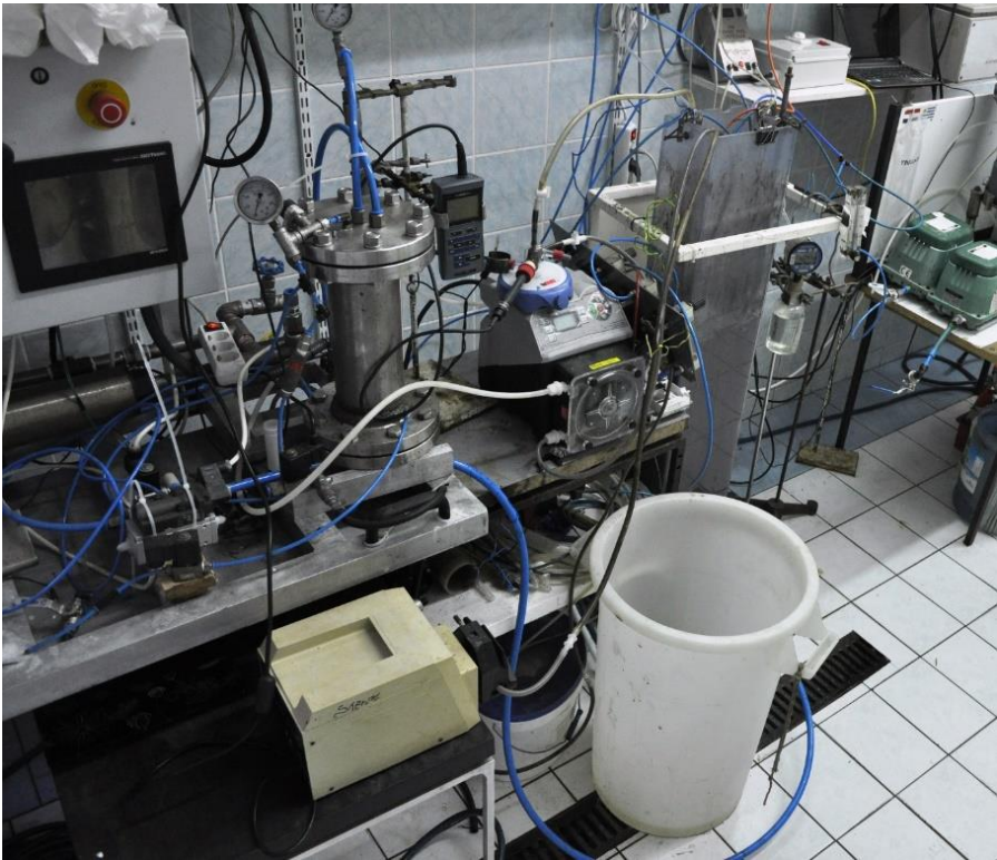
Figure 5.7 MBR-SDOX setup (Photo by Sang Yeob Kim)
