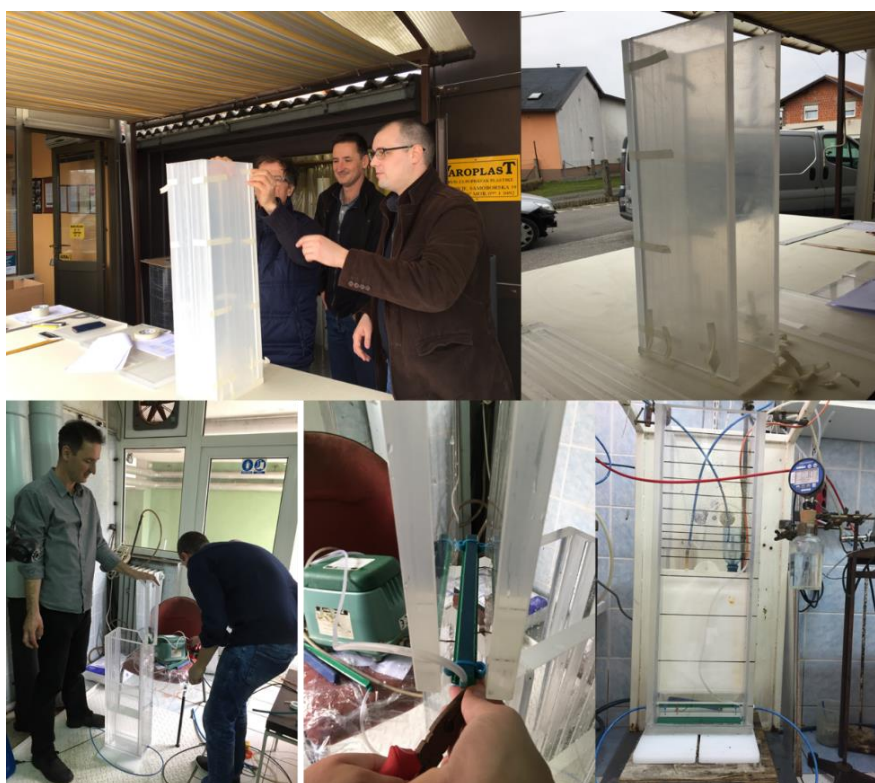
Figure 5.3 Preparation of a lab-scale membrane bioreactor (MBR) (Photo by Sang Yeob Kim)
