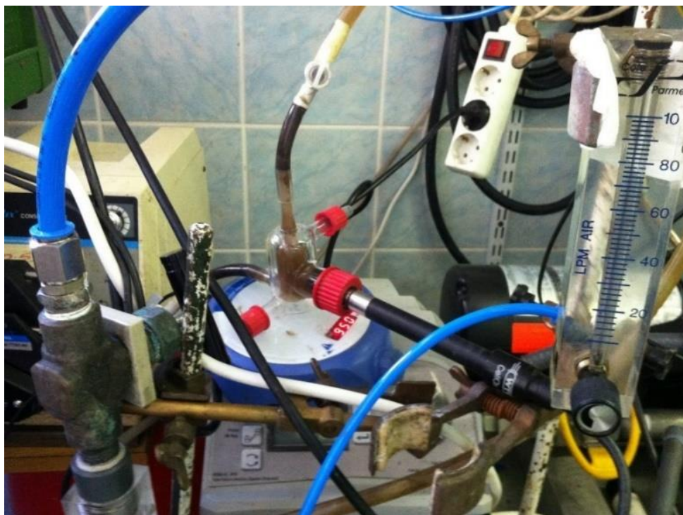
Figure 3.1 Biological oxygen meter experimental set-up for OUR determination (Photo by Sang Yeob Kim)
