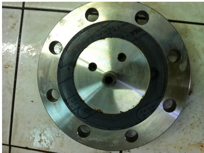
Figure 4.5 Upper part of SDOX pressurized chamber with 6 mm orifice
