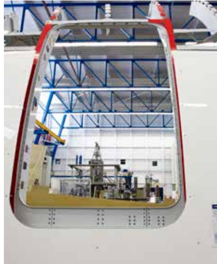
Fig. 9: Fiber Metal Laminate GLARE. – CC-BY TU Delft.
