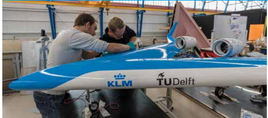
Fig. 29: The model of the Flying V in our Scaled Flight Testing Lab. © Prof. dr. H.G.C. Werij (dean) - Published with Permission
