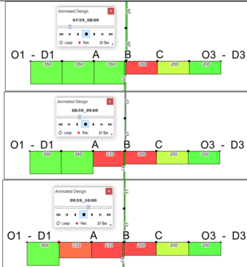
Figure 147: Flow propagation values in links of the urban intersection network_3.2.3_eGLTM
