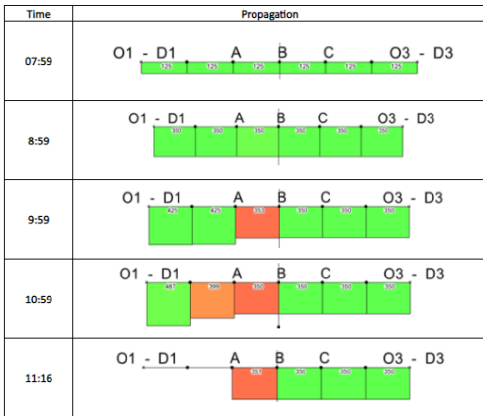
Figure 111: Flow propagation values in links of the urban intersection network_3.1.1_MaDAM
