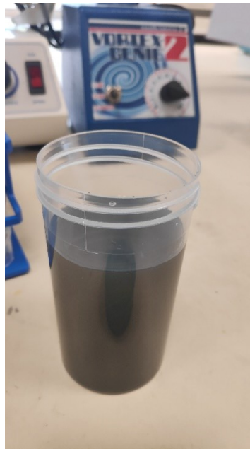
Figure 65 Image of The Final Solution Just After Electrolysis of The Municipal Effluent at an Applied Current Density Of 100 A/m 2
