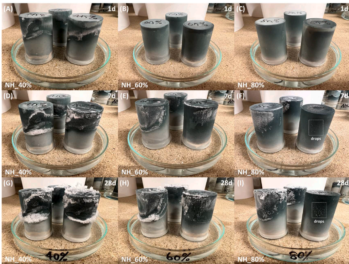
Fig. 9. Visual observation of efflorescence of NH cylinders subjected to different RH conditions of 40 %, 60 % and 80 % for 1, 7, and 28 d. The labels “NH_40 %”, “NH_60 %” and “NH_80 %” indicate the NH paste subjected to the RH of 40 %, 60 % and 80 % conditions at 20 °C, respectively.
