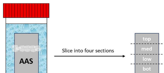
Fig. 3. Sample preparation before paste characterizations. The 7 d sealed cylinders after 28 d of efflorescence under ambient conditions are first ultrasonically cleaned, and then are sliced into four sections, designated “bot”, “low”, “med” and “top”.
