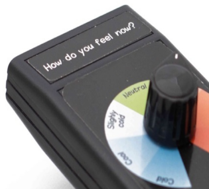
Fig. 1. Hard copy log book for entry of qualitative data and comfort dial used to capture perceived comfort levels of tenants during the Ecommon study.
