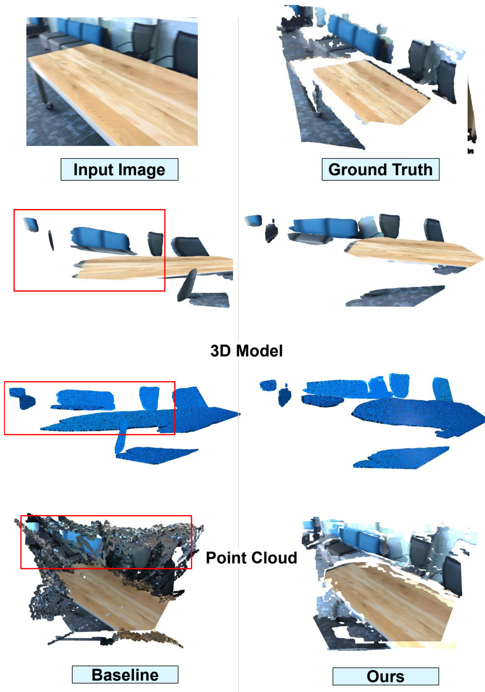
Figure 5.9: Comparison of piecewise planar model and point clouds from our model and baseline. It can be observed that in the 3D models, the table in baseline is reconstructed wrongly and goes inside the chairs while in our case, there is a clear boundary and good orientation of planar surface.
