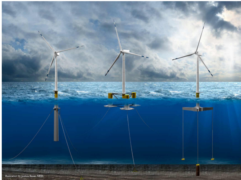
Figure 1.4: Illustration of the three basic types of floating platforms for FOWT. Source: Josh Bauer, NREL.
