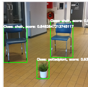
(a) YOLO detections of objects in the testing environment. Two chairs and one potted plant were detected by the algorithm.
