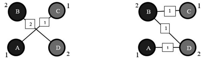
FIGURE 2 Two possible configurations to connect sources [A,B] (with given supply [1,2]) to sinks [C,D] (with given demand [1,2])
