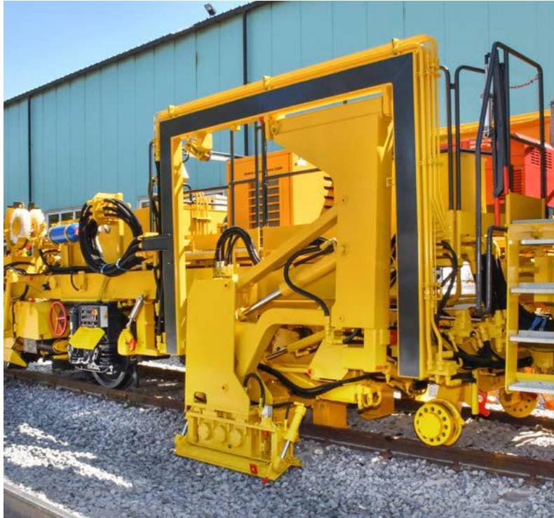
Figure 15 Crib and shoulder ballast compacter (reproduced from [74, 85])
