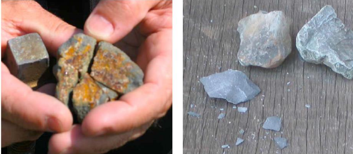
Figure 7 Ballast breakage due to tamping (figure reproduced from [18])
