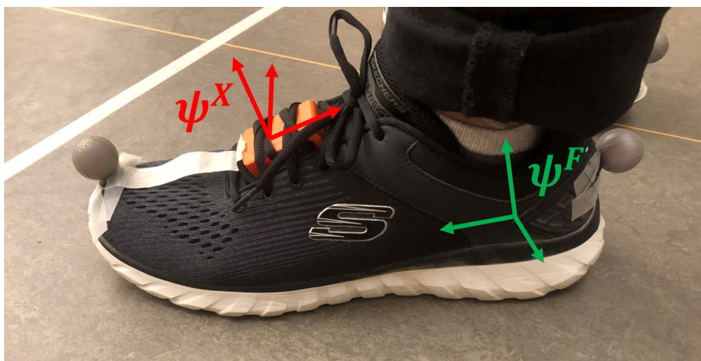
Fig. 3 Measurement setup. An IMU is secured under the shoelaces and its' coordinate system ( \psi^X ) is displayed in red. The retroreflective markers are places on the second metatarsal and the calcaneus, which is assumed to be a FPA of 0°. The foot reference coordinate system is shown in green ( \psi^F )
