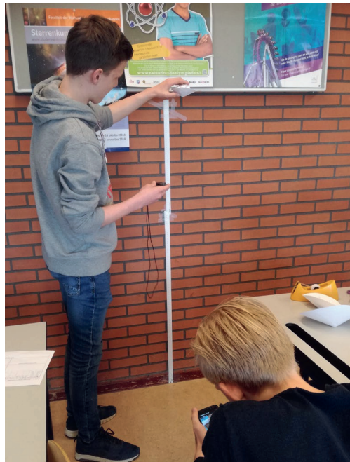
Figure 4.6. Students drop paper cones with different frontal areas and measure the falling time using both a stopwatch and their mobile phone camera.
