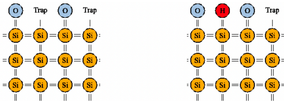
Figure 1.26: H,O chemical passivation
