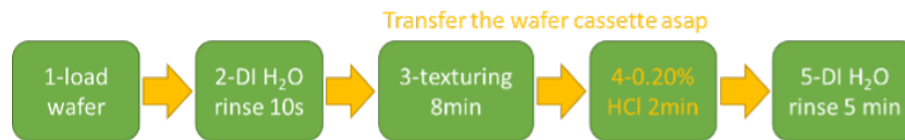
Figure 2.13: Flowchart of texturing process
