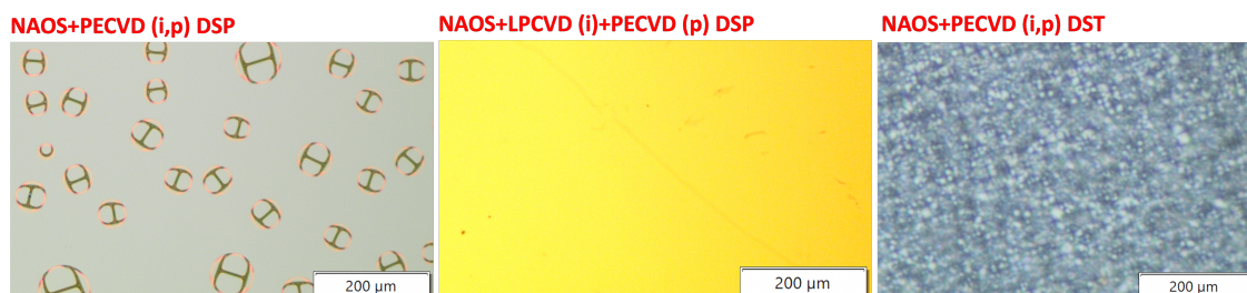
Figure 3.14: Blistering conditions of different structures observed under optical microscope.
