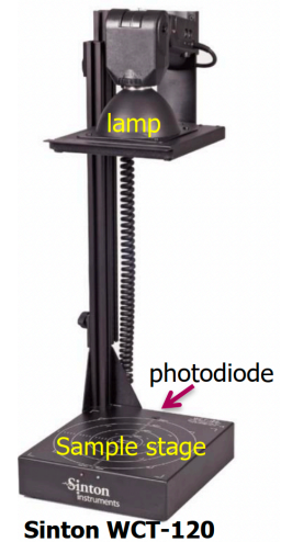
Figure 2.21: Simple schematic of Sinton WCT-120 Photoconductive Decay Lifetime Tester
