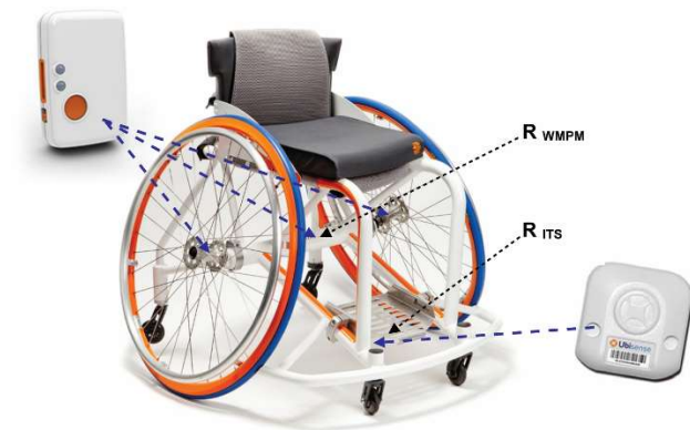
Figure 9.1: Wheelchair measurement setup, with the Ubisense tag (ITS) mounted on the footplate and the Shimmer3 inertial sensors on frame and wheels. The reference point for the ITS ( R_{ITS} ) is the same as the tag, whereas the reference point for the WMPM ( R_{WMPM} ) is the frame centre. The WMPM2 reference point is in the middle of the footplate, so close to the R_{ITS} .
