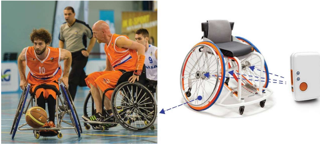
Figure 6.1: Measurement setup, with inertial sensors on wheels and frame and measurements during a match. (Photograph by www.frankvanhollebeke.be ).
