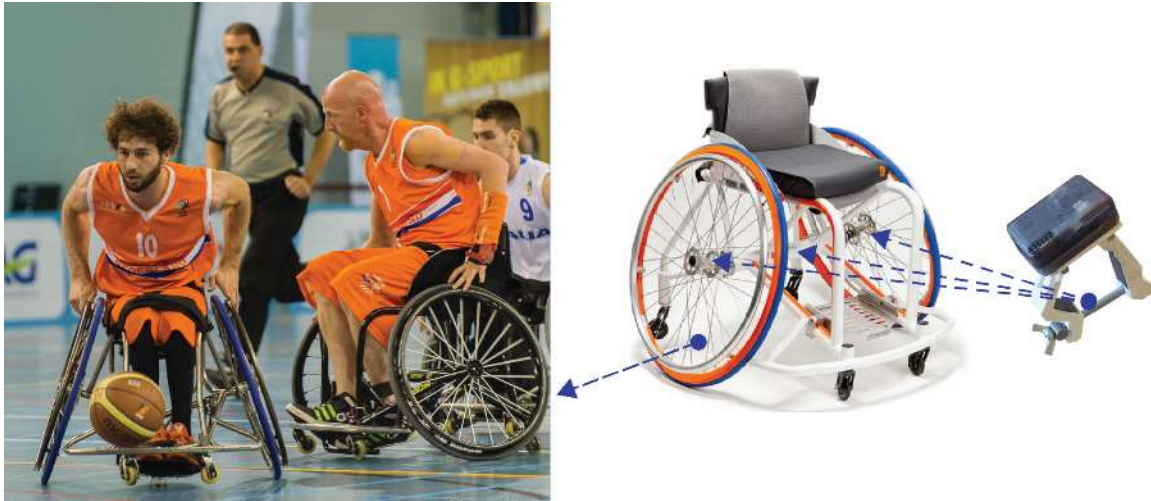
Figure 4.1: Measurement setup, with IMUs on wheels and frame and measurements during a match. (Photograph by www.frankvanhollebeke.be ).
