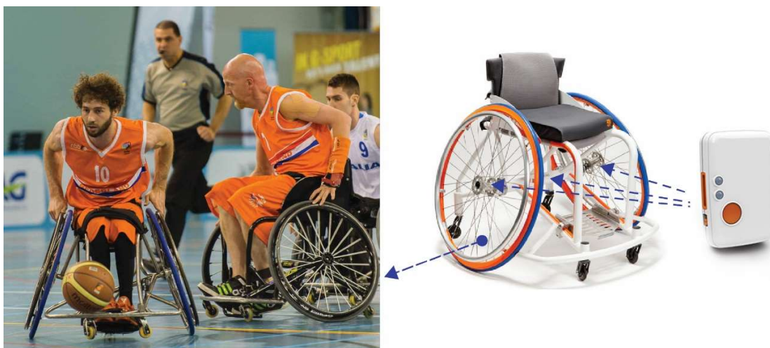
Figure 1.2: Inertial Measurement Units (IMUs) placed on the wheelchair during match play (Photograph by www.frankvanhollebeke.be ).
