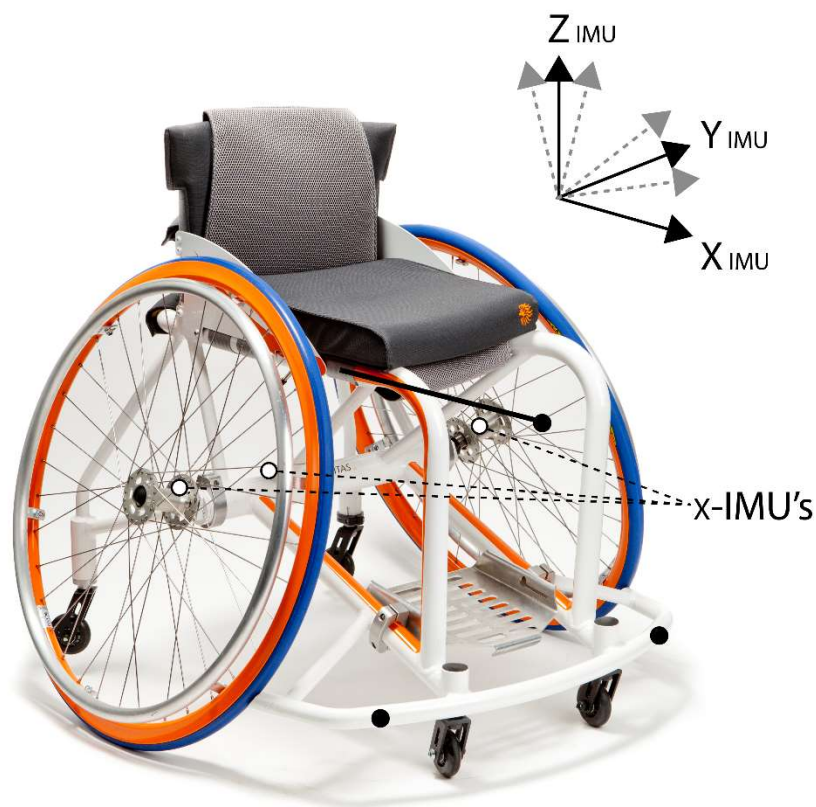
Figure 2.1: Celeritas 300 wheelchair used in the experiment. Dots indicate the position of the IR-LED markers (one on a rod). Arrows point at the locations of the x-IMU sensors. Orthogonal axes indicate x-IMU orientation at starting position for all x-IMU's, with the dashed arrows indicating the slightly rotated orientation of the wheel xIMUs due to the wheel camber angle. Mind the effect of wheel rotation around the Y-axis on x-IMU orientation.
