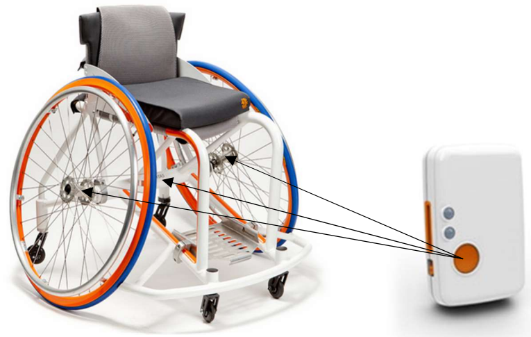
Figure 10.1: Sensor mounting locations on the wheelchair
