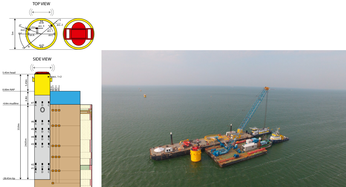
Figure 2. Left panel: measurement setup for pile W27. The orange boxes indicate the positions of the cones equipped with accelerometers and pore water pressure meters. The hatched spots on the pile (named A-D-C) indicate the position of the strain gauges, with their ring number indicated at the left side of the pile. A borehole classification of the soil is given in the right side of the figure, with yellow indicating sand, green for clay and brown for peat. Right panel: aerial photo showing the shaker on pile W27, the mobilized barges and crane.
