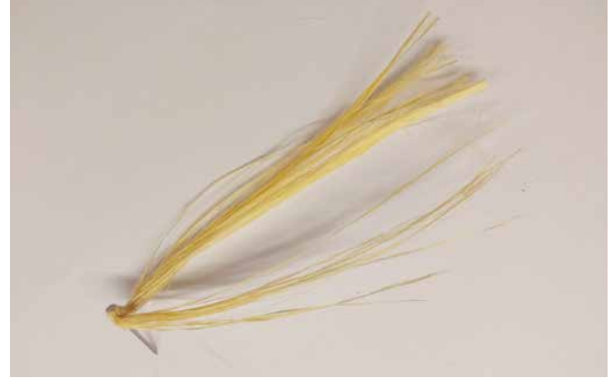
FIG. 12 Hemp gauze (left) and nails with attached hemp fibres (right): both are used to limit shrinkage cracks in the earth wall
