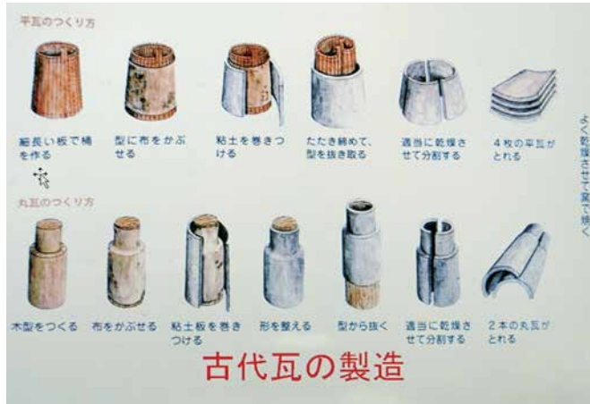
FIG. 17 Tile production in the past, with two pieces folded round a mould
