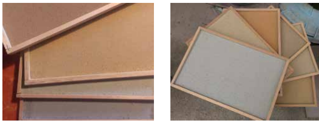
FIG. 7 Different coloured clay finishes
