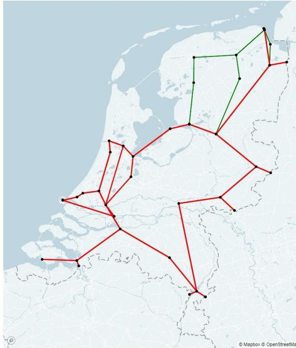
**Figure 3.1:** Depiction of the Dutch aggregated grid represented by the Dutch-HV-Power-System model. Green and red represent the 220 kV and 380 kV systems respectively. Obtained from [8]
