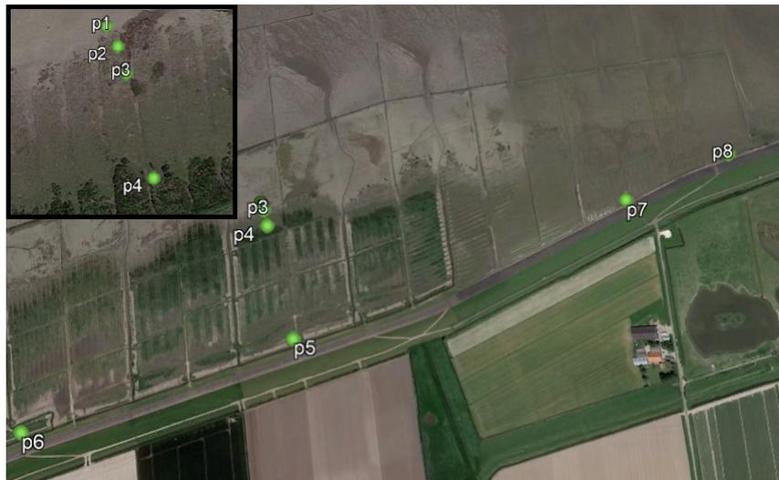
Figure 5.3: Position of the eight deployed pressure sensors at the study site during the storm of January 2015. (Modified from data provided by Vincent Vuik)
