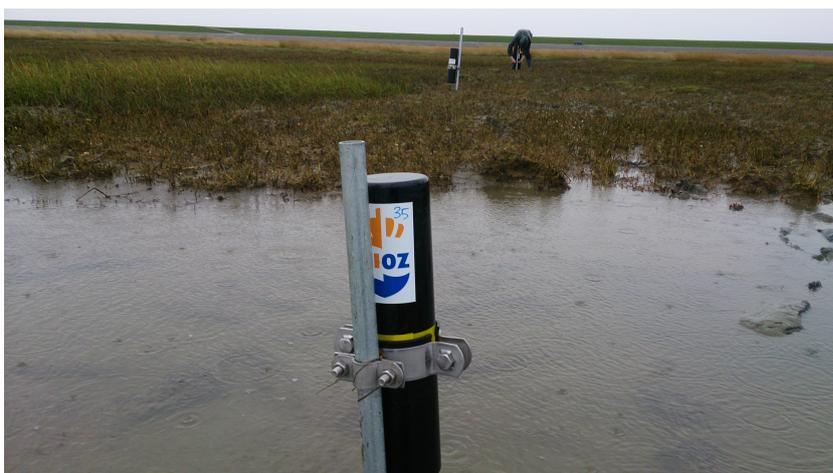
Figure 5.2: Wave gauges owned by NIOZ at the transect of study, after the storm of January 2015. On the picture is observed p1 located 2.5 m before the marsh edge, while p2 and p3 on top of the pioneer zone. Denser vegetation in the mature zone is observed closer to the dike. (Data obtained from Vincent Vuijk)
