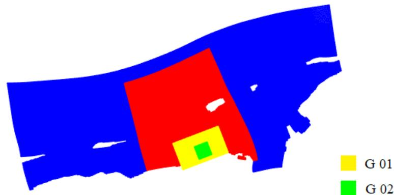
Figure 5.13: Computational Grids used for SWAN nested modeling on the research site. G01 and G02 were used during the validation and comparison investigation of this report. (Data obtained from project input files and Steetzel et al. [2018]).
