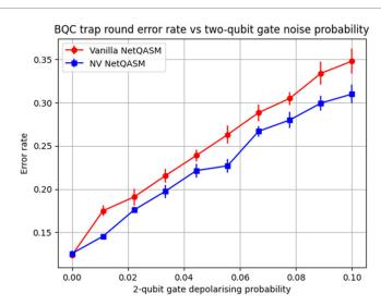
**Figure 13.** Average error rate of trap rounds for the circuit of figure 12. Each point is the average over four combinations of  $\theta_1$  and  $\theta_2$ , each used in 500 trap rounds. It can be seen that using the vanilla (platform-independent) NetQASM flavor results in a worse (higher) error rate on average.
