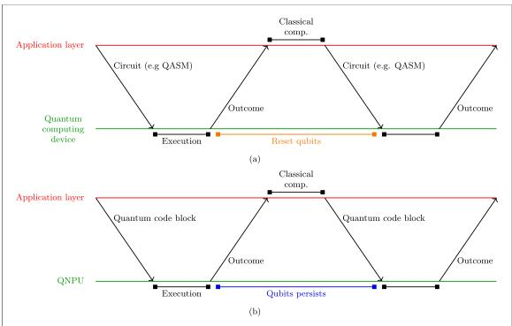
**Figure 5.** Program interaction between the application layer and a quantum device in both the case of *hybrid-quantum computing* (figure 5(a)) and quantum networks (figure 5(b)). In the case of hybrid-quantum computing, qubits are reset in between circuits (in e.g. QASM). For quantum internet programs the qubits should on the other hand be kept in memory, since they might be entangled with another node and intended to be used further.
