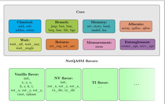
Figure 9. The core of NetQASM consists of eight groups of instructions. The quantum gates are defined as a set of software-visible gates part of a NetQASM flavor. The vanilla flavor is the unique platform-independent NetQASM flavor of NetQASM, which can be used by a compiler.
