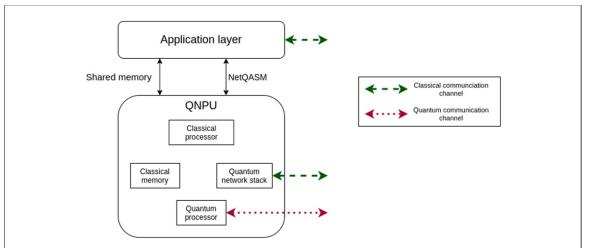
**Figure 4.** Overview of QNPU components and interfaces. The application layer talks to the QNPU using NetQASM. The processor inside the QNPU can interact with all other components. Channels are connecting components with corresponding components in adjacent nodes in the network.
