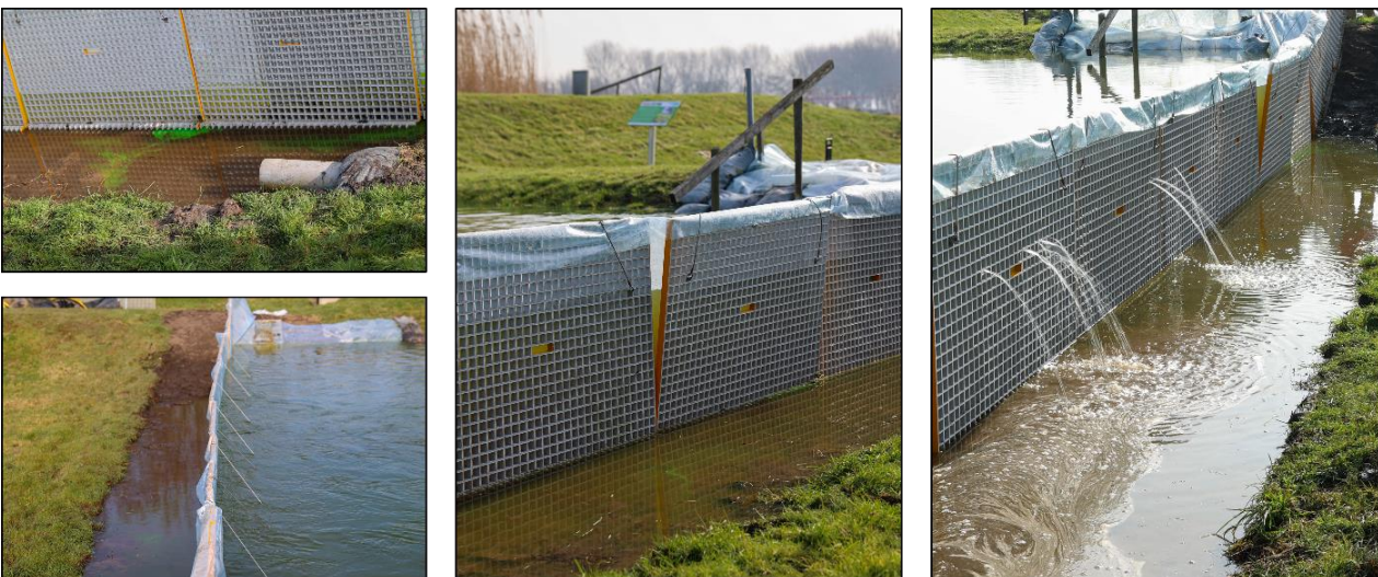
Figure 23 Water retention capacity test of H-Wall
