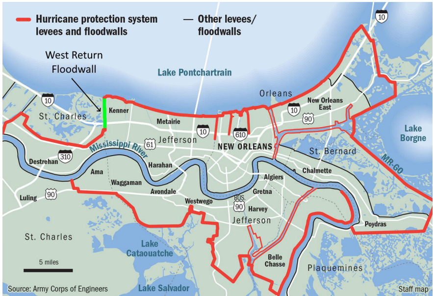
Figure 31: The HSDRRS flood protection system of New Orleans, with the West Return Floodwall indicated in green (adapted from Swenson, 2022)
