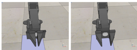
Fig. 14. Left and right figures show the closed and open positions, respectively, of the PhantomX robot gripper.
