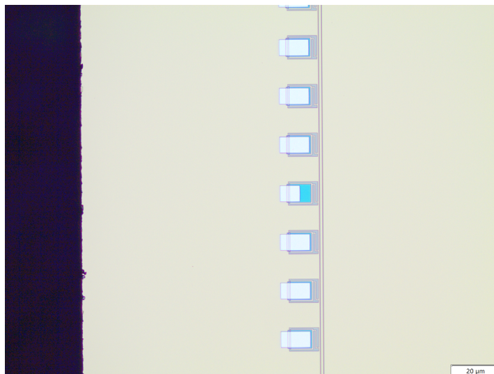
Figure 3.28: Here we see seven resonators. The middle one is designed to have a different resonance frequency. The Al covers only the half of the dielectric area thereby creating a capacitor with a halved capacitance compared to the other ones.
