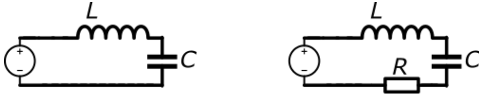
Figure 2.3: Circuit diagrams of a series (left) LC oscillator and (right) LCR oscillator.
