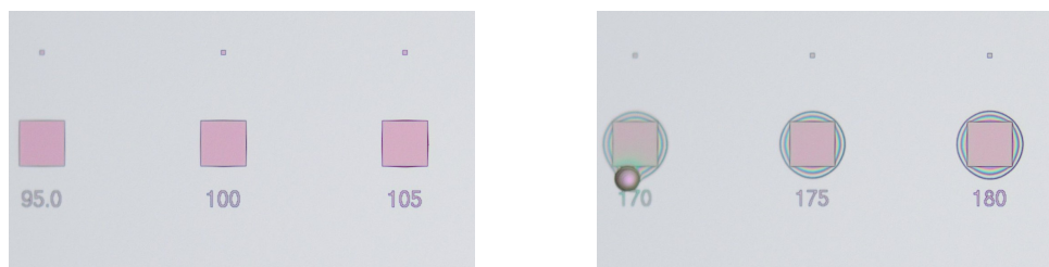
Figure 3.16: Images taken from an optical microscope. The numbers under the pink squares represent the doses in \mu\text{C}/\text{cm}^2 . We found 100 \mu\text{C}/\text{cm}^2 to be the right dose (left). The right image shows how the squares look after over exposure.
