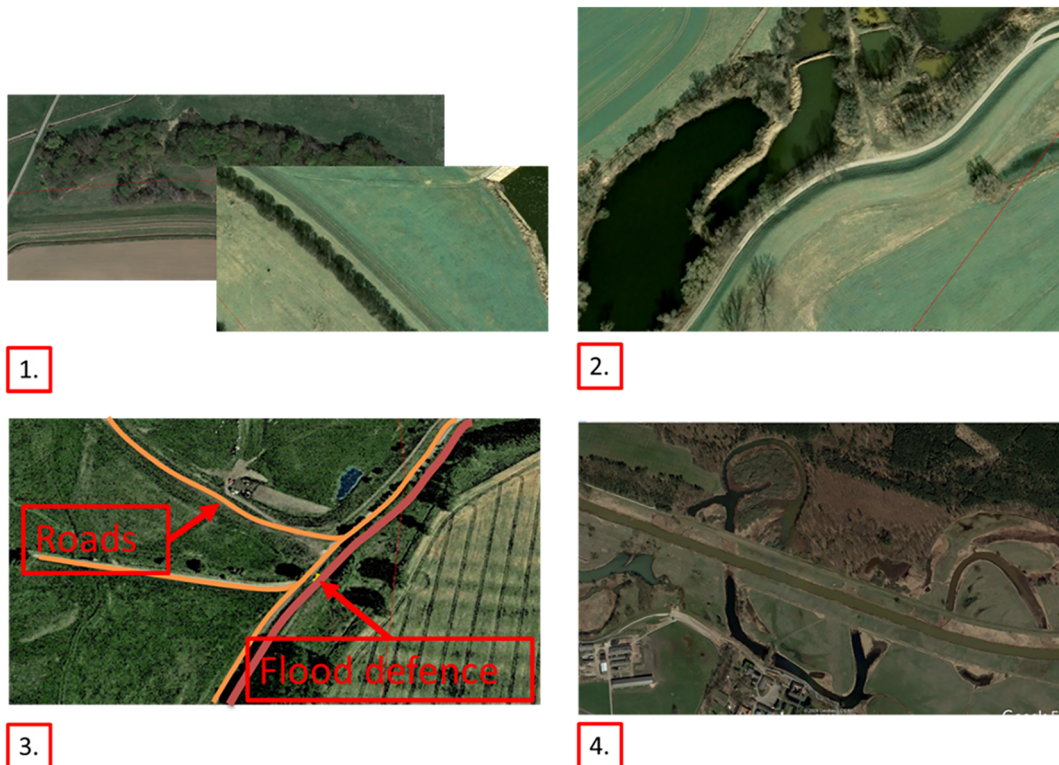
FIGURE 8 Illustration of deviating conditions (samples were taken from the Sachsen-Anhalt river system (Google, 2020a), 1: bushes or trees next to the levee, 2: permanent water directly next to the levee, 3: geometric changes of the cross-section of the levee (the road in orange on the levee in red branches off with several turns toward the river), 4: geological deviation observable in the subsurface, for example, old river belts
