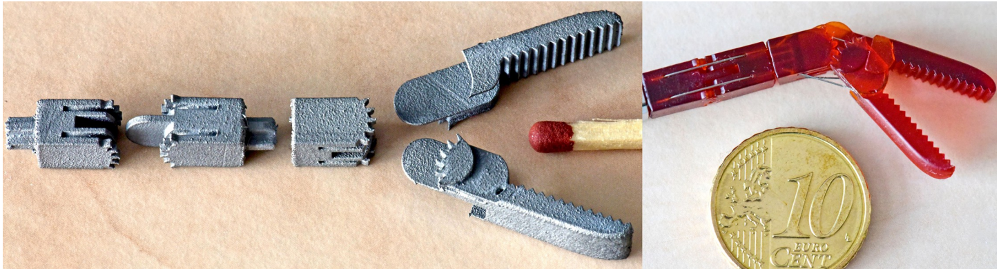
Fig 1. Example showing the rough surface of parts printed with metal additive manufacturing (left). The parts are meant to be used in a steerable, medical instrument, however they require extensive polishing before they can be used in a functional mechanism. The match is shown for scale. As comparison, on the right the same parts 3D printed using a polymer-based additive manufacturing process.
