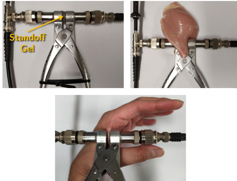
FIGURE 15. Mediums/Phantoms employed: Standoff Gel (top left), chicken breast (top right) and human hand (bottom).
