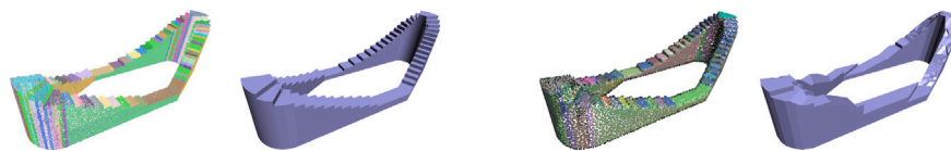
Fig. 22. The impact of the quality of detected planar primitives on the final reconstruction. Left: given accurately detected planar primitives, our method reconstructs high-quality building models. Right: the reconstruction result from inaccurately detected planar primitives.
