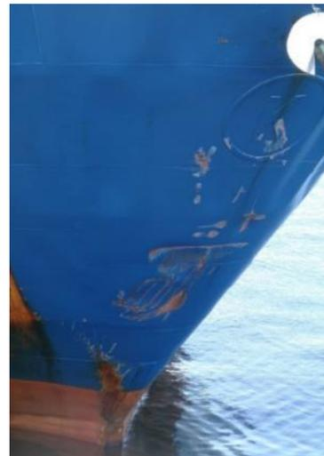
(b) Damage to the "Else's" bow above the waterline
