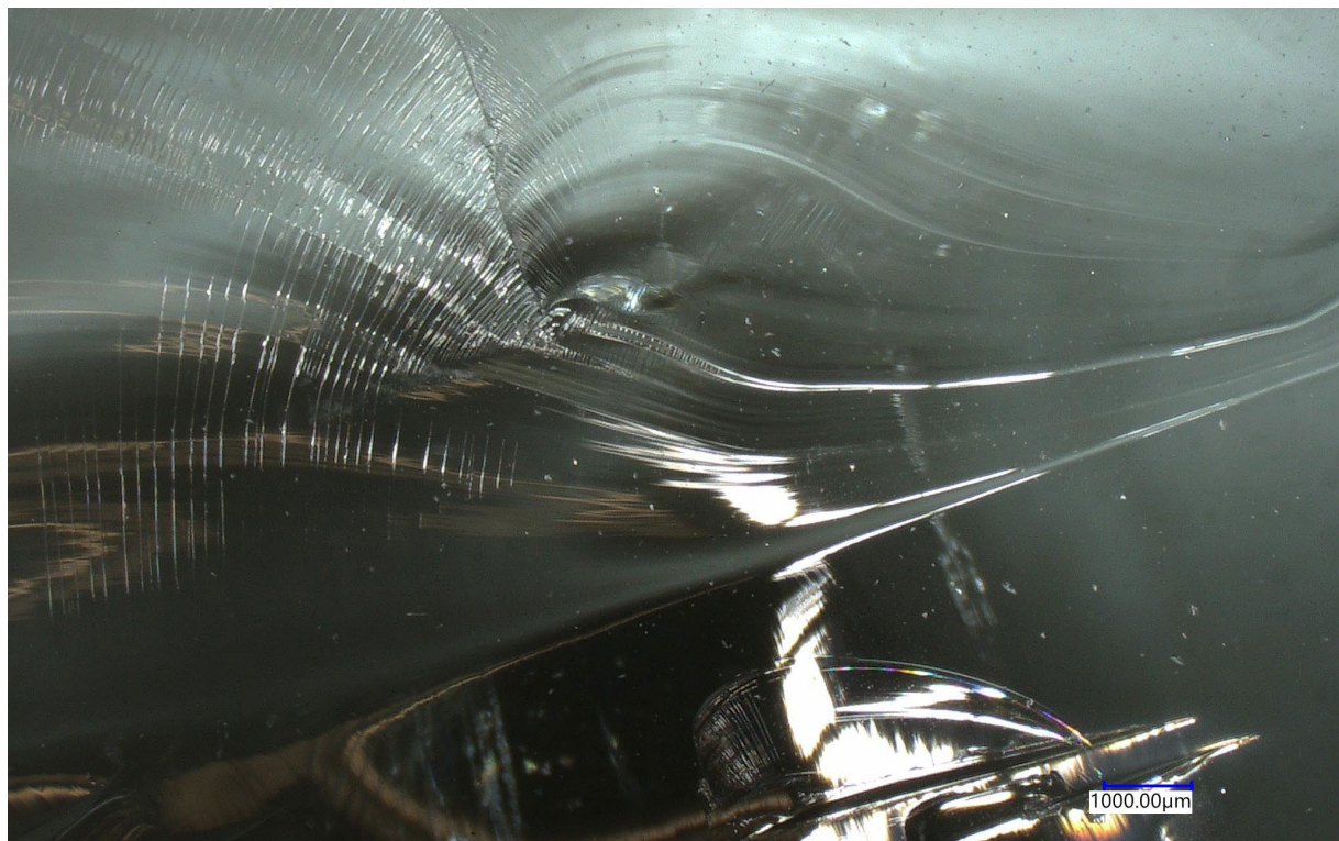
Figure 88 Shear marks of trial test run sample 4
