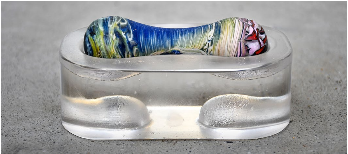
Figure 16 Doggy bone interlocking brick (Oikonomopoulou et al., 2018)
