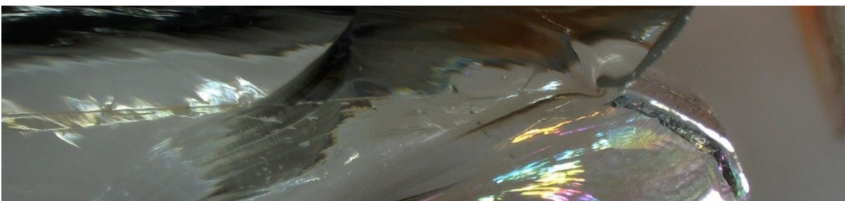
Figure 61 Close-up of fusing surface line in 3 hour beam (Bristogianni et al., 2020)
