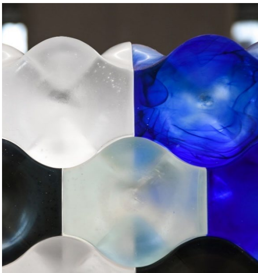
Figure 14 Osteomorphic interlocking bricks (Oikonomopoulou et al., 2018)
