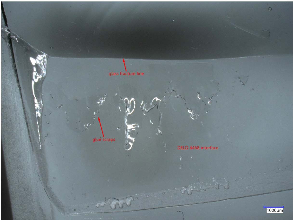
Figure 97 Failure surface of sample DELO 1
