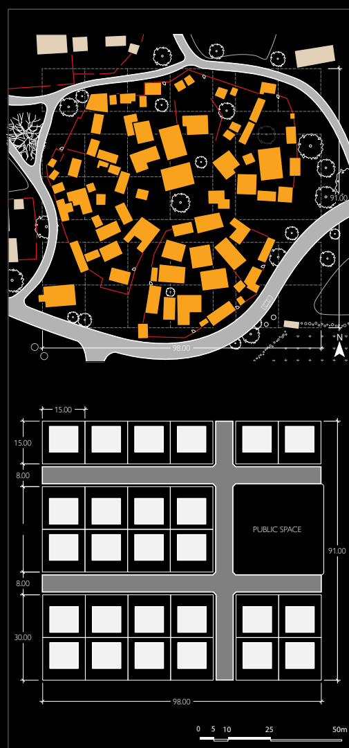
Figure 2. Top: Fojn compound in Kholpa. This is a recognizable Sérère type of compound. Bottom: The spatial plan for the expansion in Kholpa.
