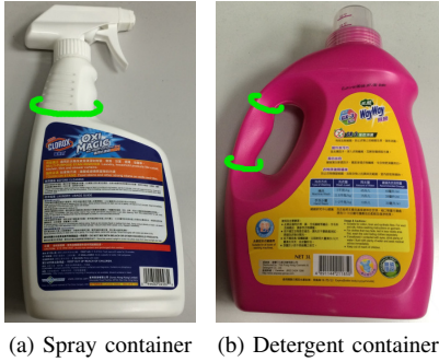
Fig. 9. Two objects for evaluating the performance of rope grasping on a spray container and a detergent container. The spray container has a bottle-neck, while the detergent container has a handle. The candidate rope caging grasps for these two objects are marked by the green curves.
