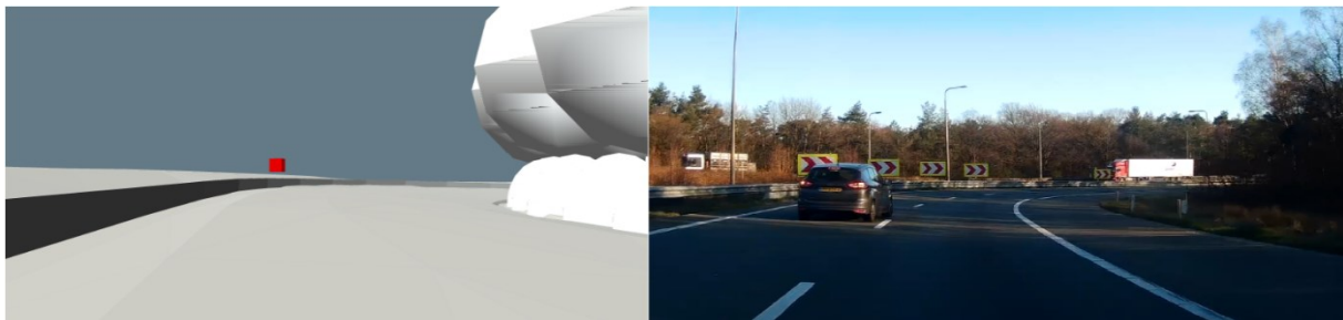
Figure 3-3 On the left the analysis of “Zicht” on the visibility of the curve signs. The red object in the 3D model is the object “Zicht” checks along the alignment, in this case a curve sign, positioned above the guardrail (the dark grey line). On the right, this exact viewpoint is shown in the real life situation.
