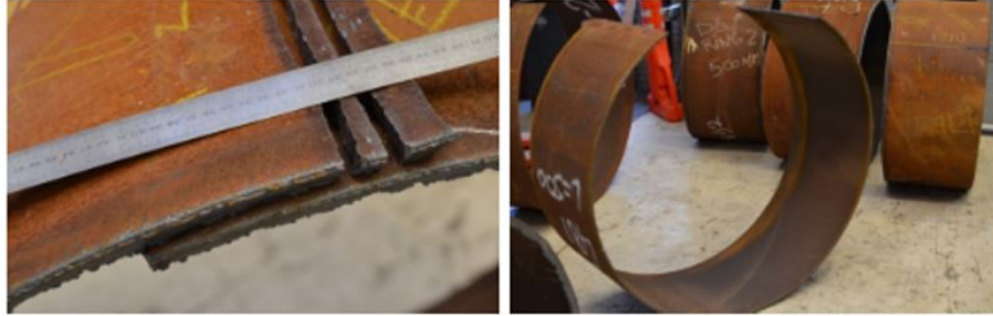
Figure 3.7: cutted ring segments from residual stress estimation S. van Es [13]
