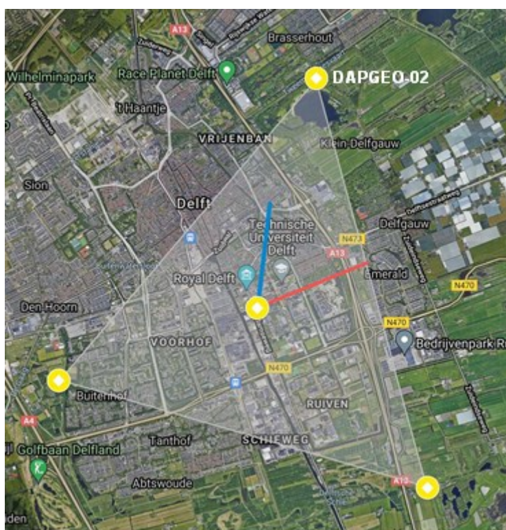
Figure 4: Layout of the local seismic geophone network (orientation such that north is vertical)
