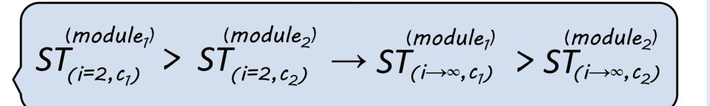
• Value of the  $ST_{(i=2,c)}$  can be used instead of  $ST_{(i\to\infty,c)}$ for comparison of shading tolerability of PV modules.
