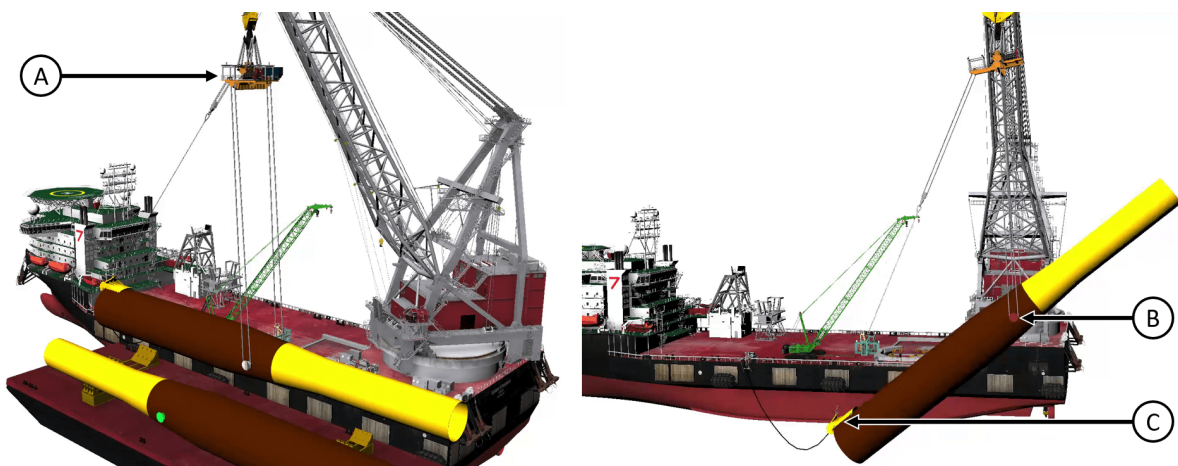
Figure 1.2: Demonstration of the working principle of the Monopile Upending Smart Tool (MUST)
