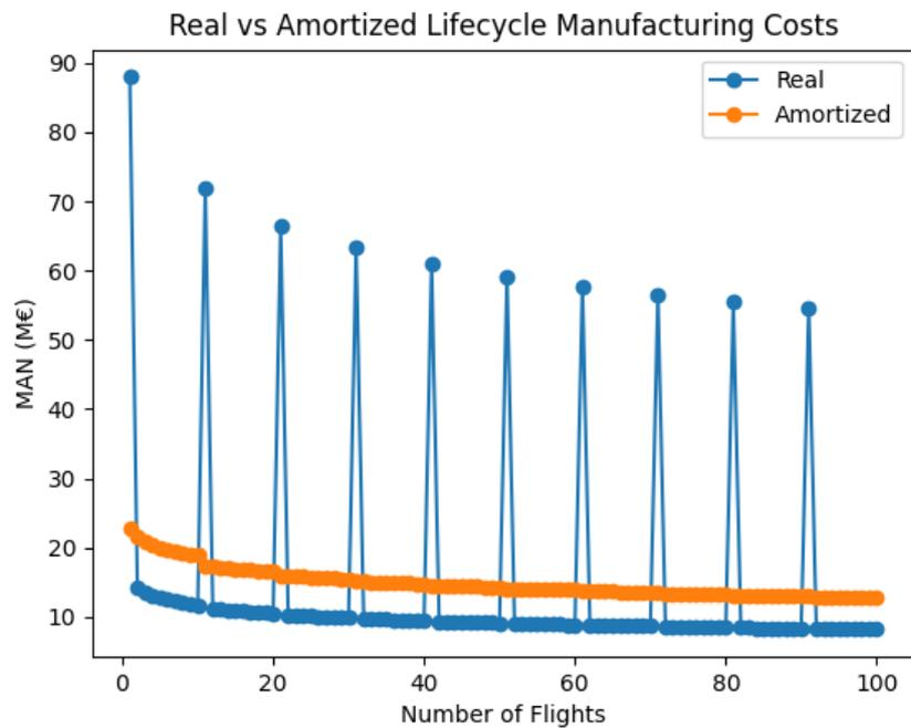
Figure 5.3: Falcon 9 manufacturing costs, comparing the real costs to the amortized version for better visualization.
