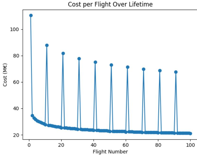
Figure 5.7: Falcon 9 Cost per Flight over Life Time
