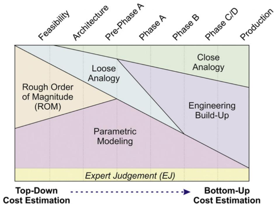
Figure 2.1: Qualitative application of CEMs according to project phase [136].
