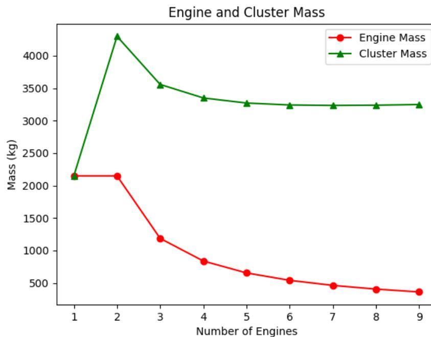
Figure 6.4: Evolution of the mass of a single engine and cluster with the number of engines in the configuration.
