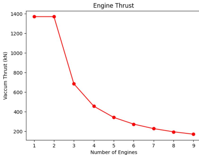
Figure 6.3: Thrust to which each engine is rated in order to enable engine-out capability.
