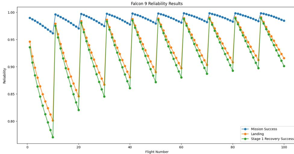
Figure 5.19: Falcon 9 reliability results, including mission and landing reliabilities, and the probability of recovering the first stage
