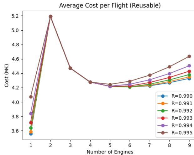
Figure 6.22: Cost per flight sensitivity to 30% higher landing mass.
