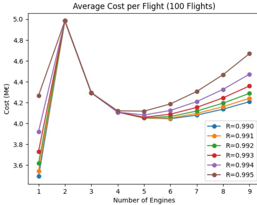
Figure 6.17: Cost per flight including engines and landing gear manufacturing and operations (including retrieval and refurbishment), for different targets of reliability.
