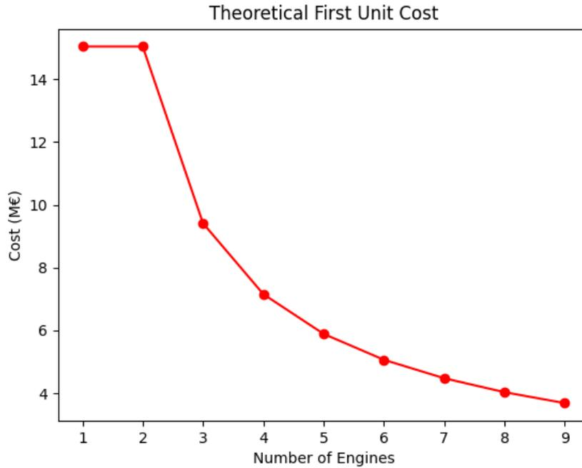
Figure 6.9: Engine theoretical first unit costs variation with the number of engines.
