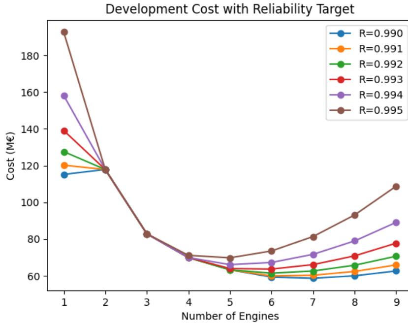
Figure 6.12: Development costs accounting for extra tests needed to reach different reliability targets.
