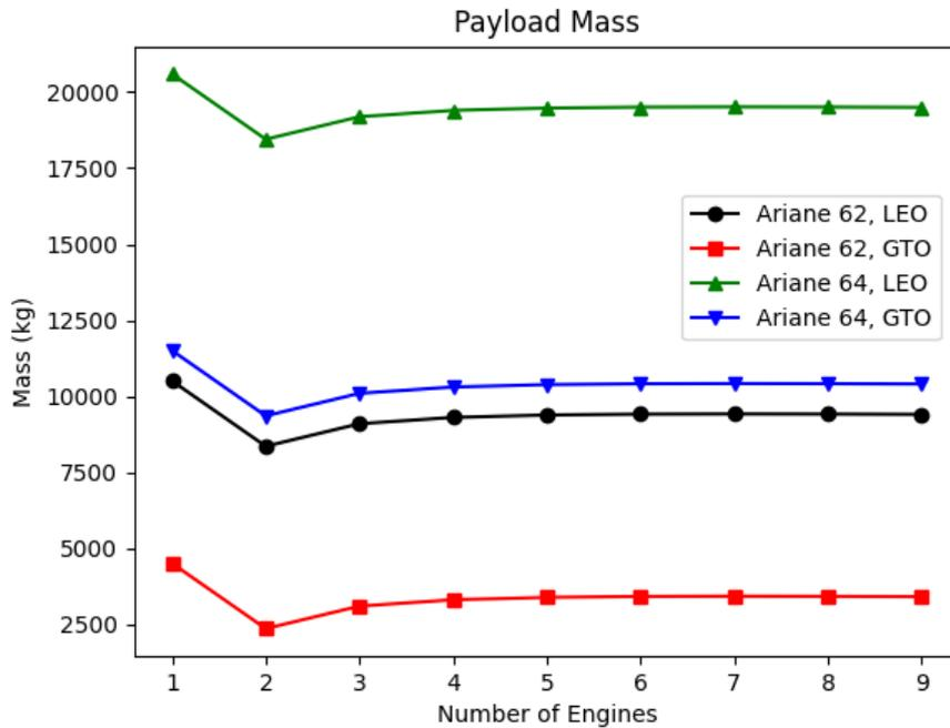
Figure 6.5: Variation of Payload Mass with the number of engines in a given configuration.
