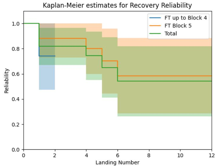
Figure 5.13: Recovery reliability estimate obtained with a Kaplan-Meier estimator (95% confidence bounds), for Falcon 9 Full Thrust up to Block 4, Block 5, and both combined
