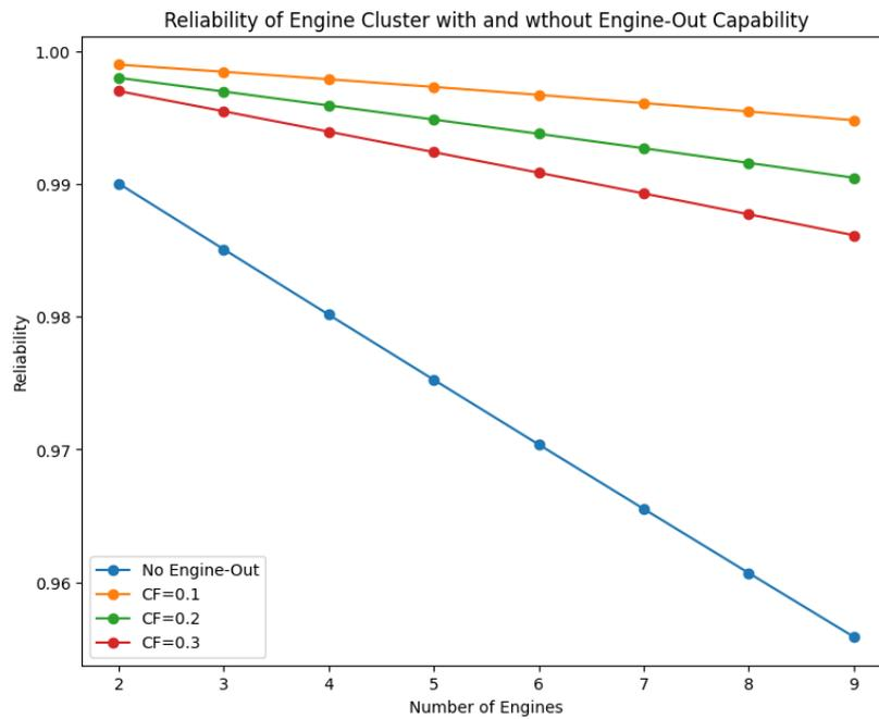
Figure 3.6: Effect of the engine-out capability, depending on the catastrophic failure percentage.
