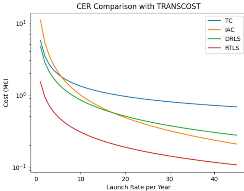
Figure 4.4: Comparison of recovery CERs with TRANSCOST model.
