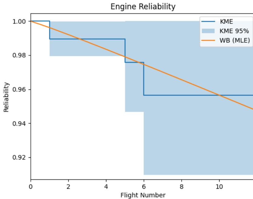
Figure 5.12: Comparison of the non-parametric estimate with KME and the parametric estimate with MLE assuming Weibull distribution
