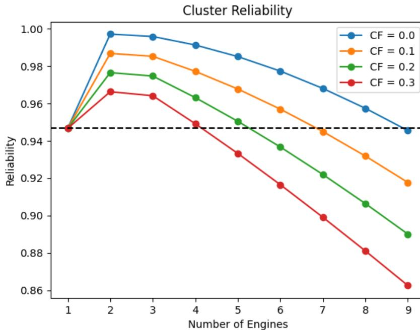
Figure 6.7: Sensitivity of cluster reliability to the catastrophic failure percentage (CF).
