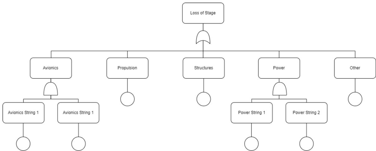
Figure 5.17: Fault Tree Analysis at subsystem level.
