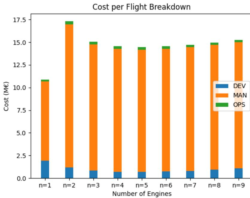
Figure 6.16: Average Cost per Flight breakdown, as a function of the number of engines in the configuration.
