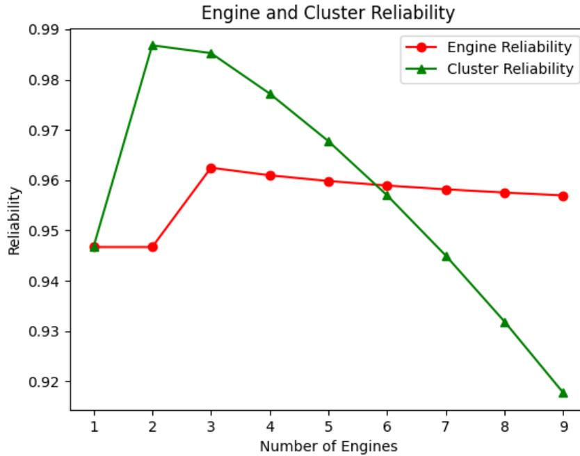
Figure 6.6: Single-engine reliability resulting from derating and engine cluster with engine-out capability reliability, as a function of the number of engines in configuration (CF=0.1).
