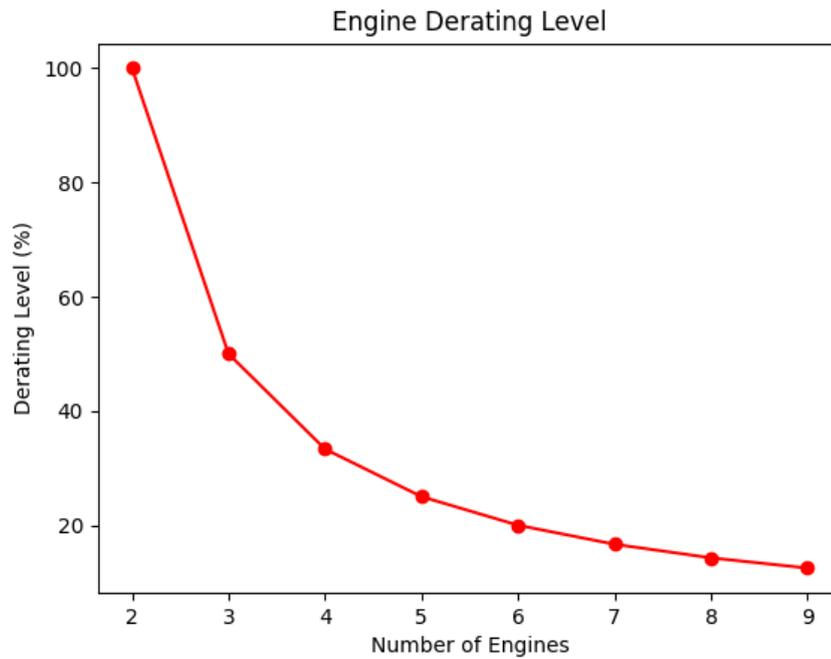
Figure 6.2: Derating level corresponding to the number of engines in each configuration.
