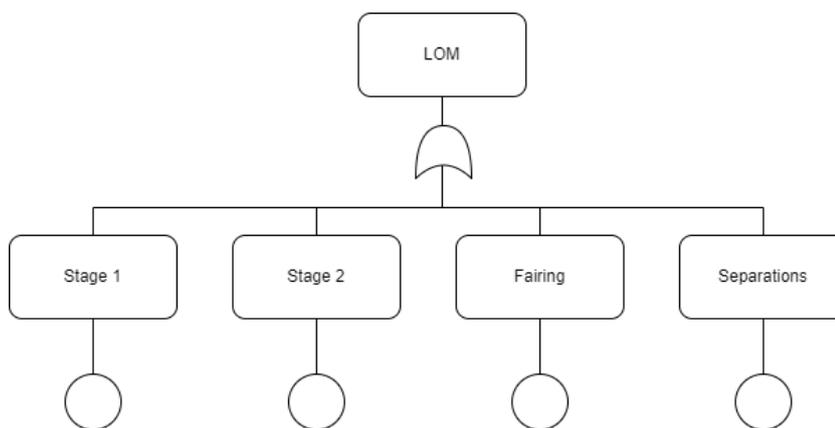
Figure 5.16: Fault Tree Analysis at stage level.
