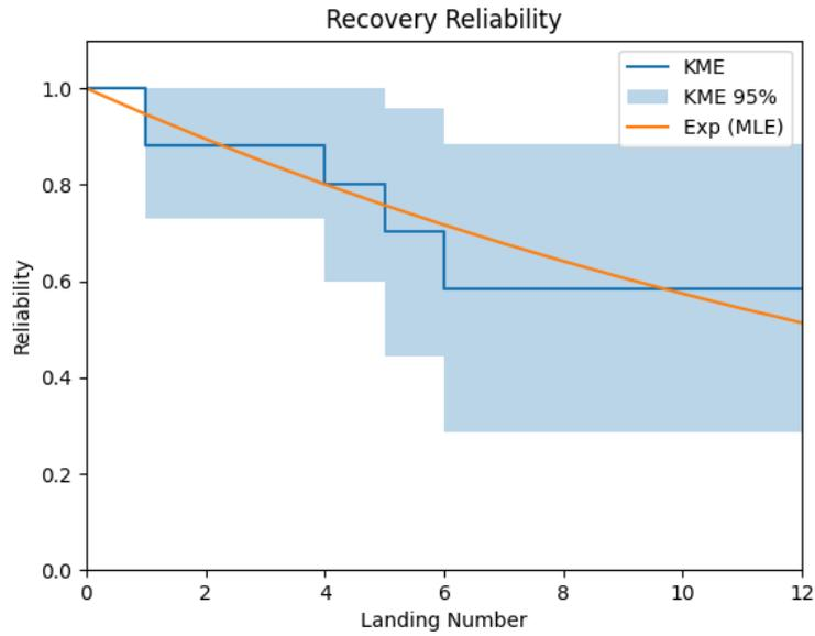
Figure 5.15: Comparison of the non-parametric recovery estimate with KME and the parametric estimate with MLE assuming exponential distribution.
