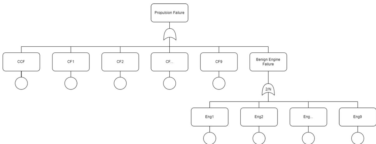
Figure 5.18: Fault Tree Analysis at engine level.
