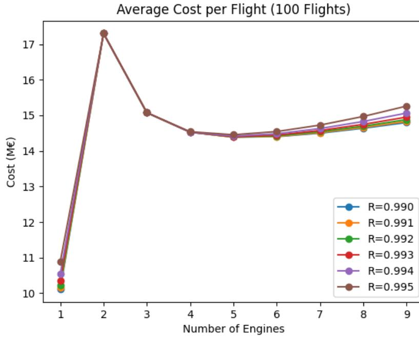
Figure 6.15: Engine manufacturing cost per flight for 100 flights
