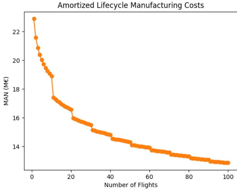
Figure 5.2: Falcon 9 manufacturing costs with amortized booster costs.
