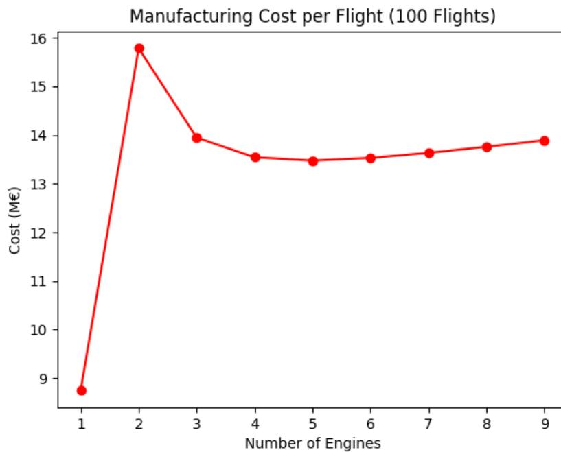
Figure 6.13: Engine manufacturing cost per flight for 100 flights
