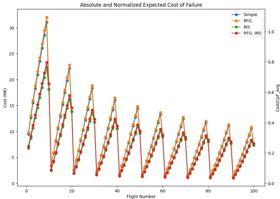
Figure 5.20: Falcon 9 absolute (left) and normalized (right) Expected Cost of Failure.
