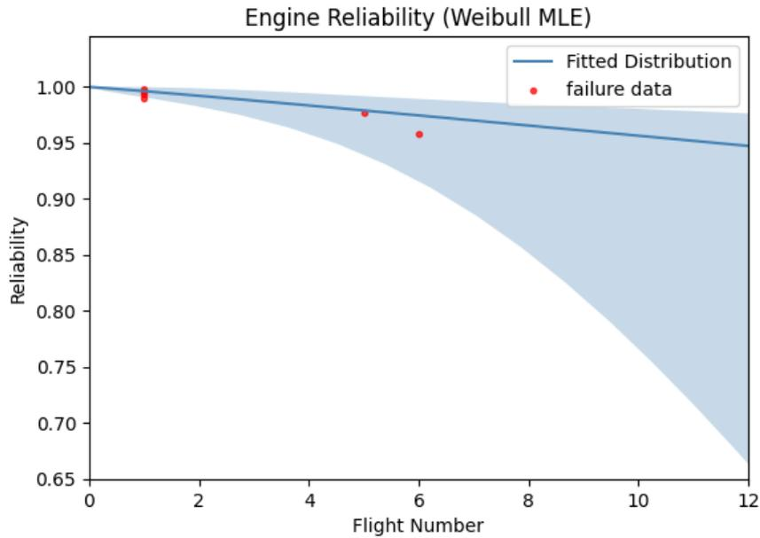
Figure 5.11: Engine reliability estimate obtained with a MLE, assuming a Weibull distribution (95% confidence).
