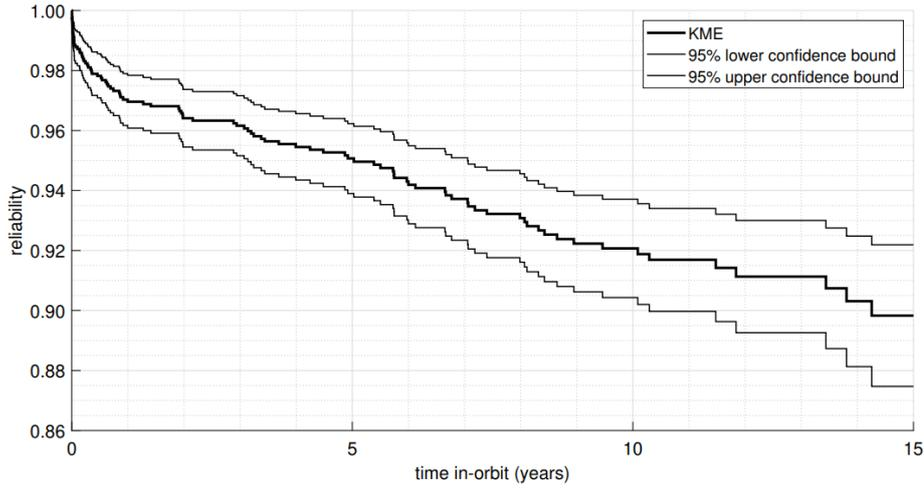
Figure 3.3: Application of a Kaplan-Meier Estimator to a satellite failure database [82].
