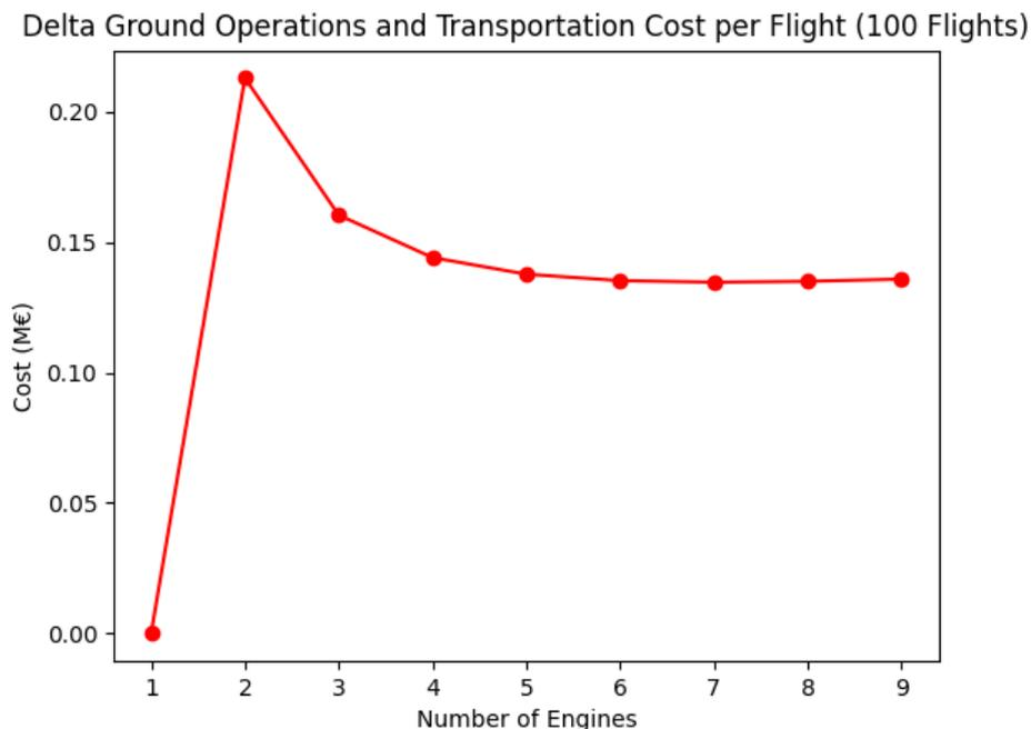
Figure 6.14: Operating cost per flight for 100 flights, pertaining only to the engine cluster.
