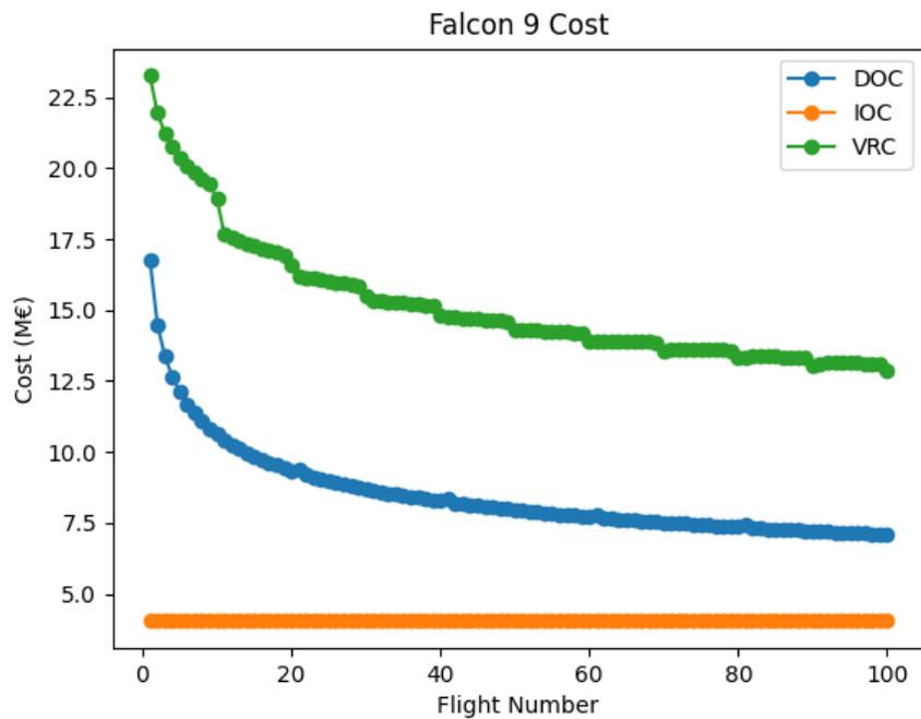
Figure 5.5: Falcon 9 operations cost with time.
