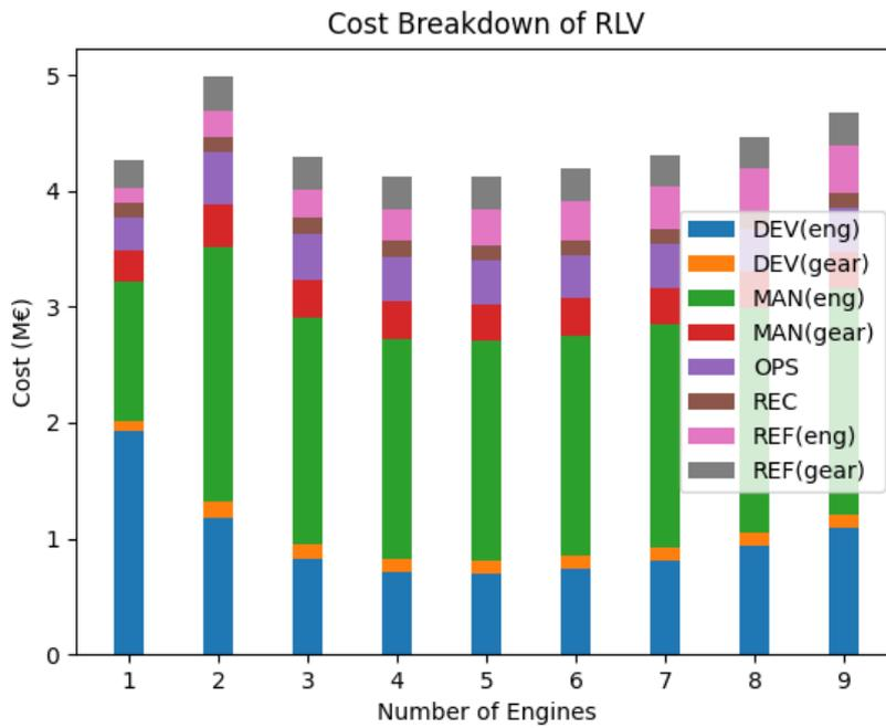
Figure 6.18: Cost breakdown for RLV with engine cluster reliability requirement of 0.995.
