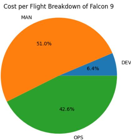
Figure 5.8: Falcon 9 estimated Cost per Flight Breakdown.
