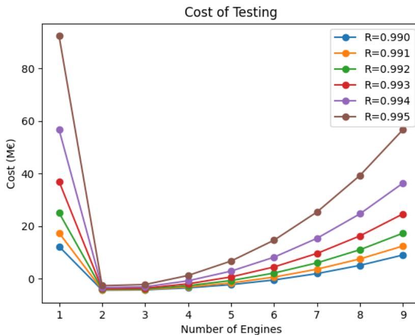
Figure 6.11: Cost of the testing needed to reach reliability targets.
