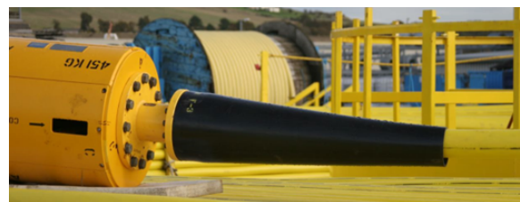
(b) Real-life bend stiffener and attachment [31]
