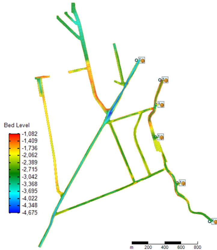
Figure 5.2: Updated bed level values (m NAP) for the van Lennep case study.
