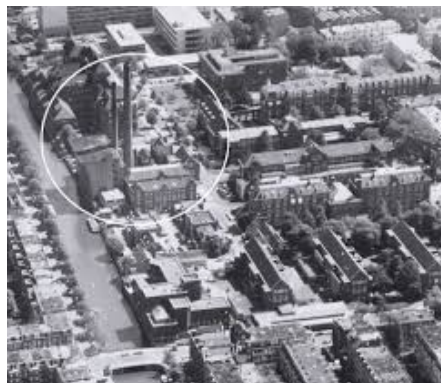
(a) The old ketelhuis (English: boiler room) at the Van Lennepkanaal (in 1973). Heat was provided to the Wilhelmina Gasthuis district by burning coal that was transported over the water. The building was demolished in 1983. (Source: beeldbank Amsterdam).
