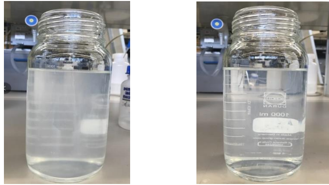
Figure 5.3 0.5g/L powder silica. Original(left), After dispersion(right)
