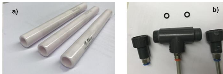
Figure 5. 2 a) ceramic nanofiltration membranes b) membrane house
