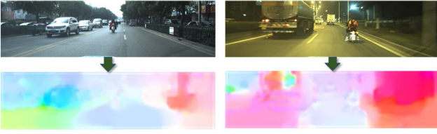
Fig. 3. Calculated optical flow image (converted to RGB format).
