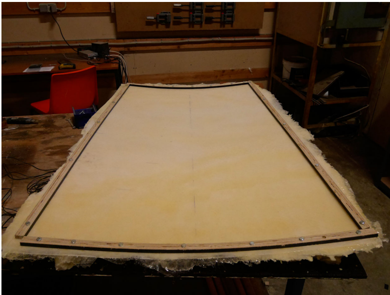
Figure 18. Fitting timber edge barriers on the mould.
