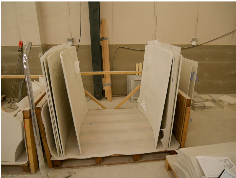
Figure 36. Finished cast panels for ring 1 and ring 2.
