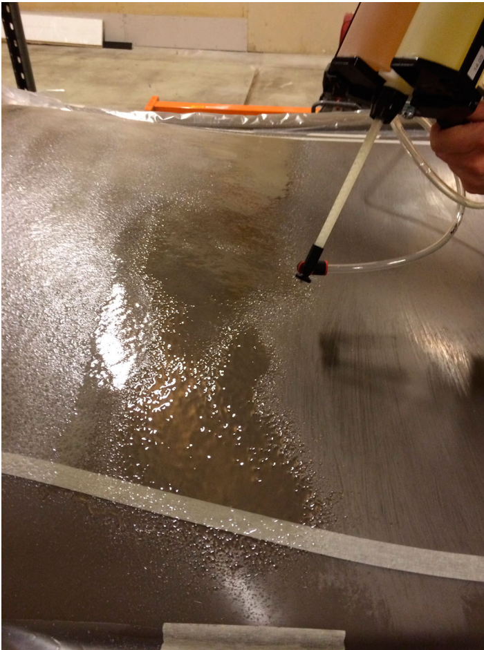
Figure 20. Applying the hard coat.
