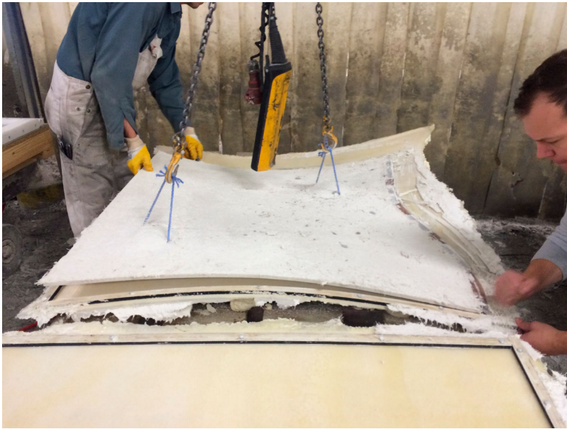
Figure 24. Demoulding of the free-form prototype.
