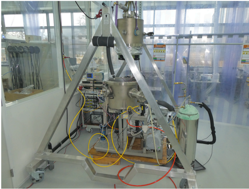
Fig. 4. Open vacuum chamber and control and measurement equipment.
