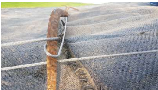
(a) Permeable geotextile.
