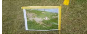
Figure 5.3: Unrealistic imitation damage grass revetment.
